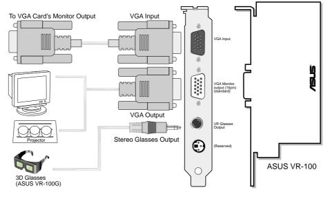
You must anchor the ASUS VR-100's mounting bracket with a screw to a free expansion slot in your computer chassis.
